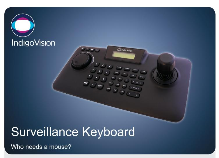
IndigoVision's Surveillance Keyboard is used to access Control Center's Virtual Matrix and IP Video Wall. The Control Center Virtual Matrix allows the Surveillance Keyboard to control IndigoVision and most third party PTZ cameras including Pelco and Panasonic.
